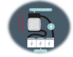
Regenerative braking captures this typically wasted energy to create electricity, which charges the battery.
